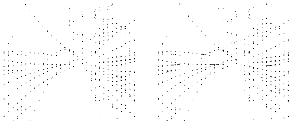
Figure 26. Event in the pixel detector, with the horizontal coordinate compressed by factor 10. Left: raw event, right: segments found at the entrance and exit of the detector.
