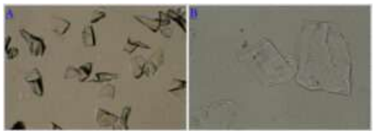
5.35 (A) Garnet showing high relief, and (B) halite showing low relief (PP light)
