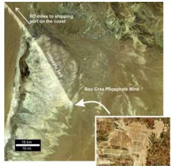
9.99 Phosphate is shipped nearly 60 miles via a covered conveyer belt from the mine in the Western Sahara to the coast where it is transported for use as fertilizer around the world.
