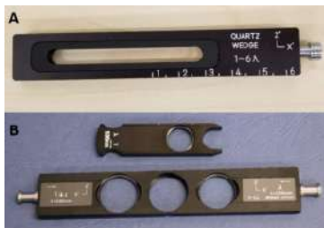
5.28 A quartz wedge (A) and two examples of accessory plates (B)
