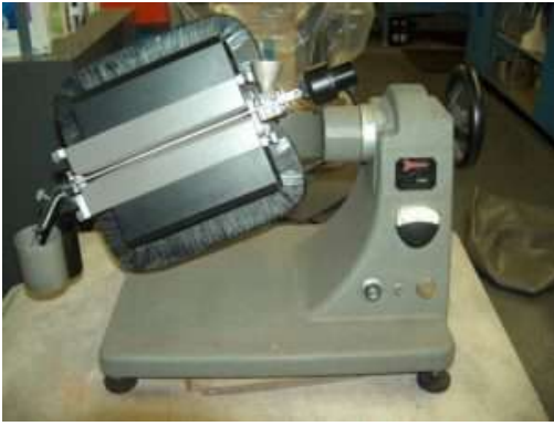
3.81 Magnetic separator for laboratory use
