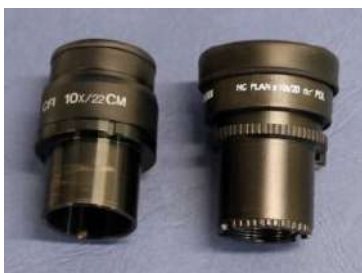
5.27 Microscope eyepieces that contain ocular lenses
