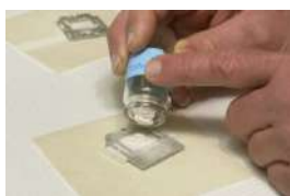
12.21 A sample holder being loaded with a powdered sample
