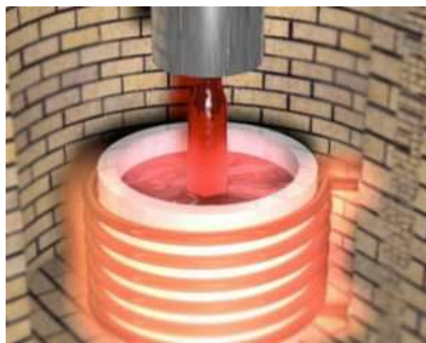
9.70 Ruby being created by the Czochralski method
