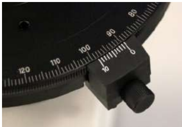
5.25 Angular scale on a microscope stage
