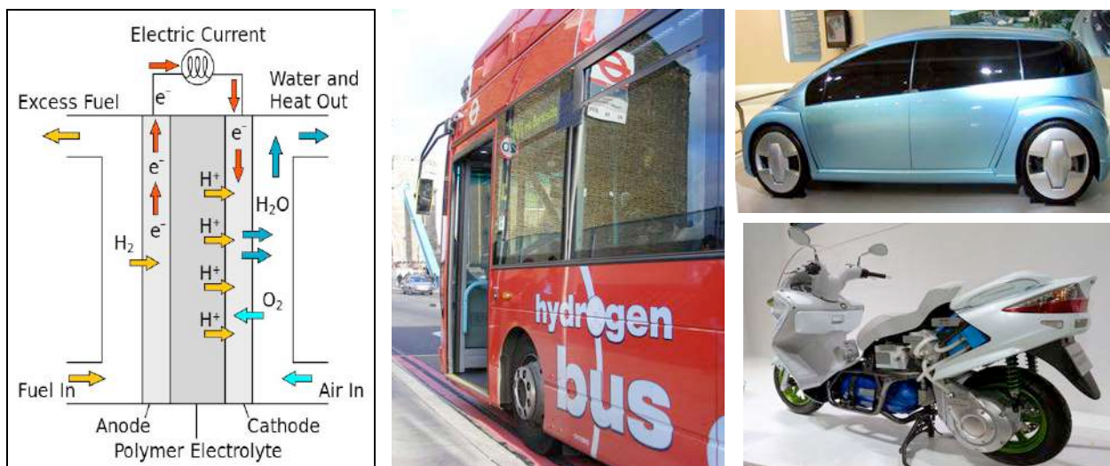
Figure 5.14: The electrochemical processes showing how hydrogen fuel is combined with oxygen generating heat energy along with water as a waste product. Some vehicles that use the fuel cell include buses (photo is a hydrogen fuel bus on Tower Bridge London, photo by Sludge G.), cars (The Toyota Fine N car based on fuel cell technology, photo by Chris 73, CC BY-SA 3.0) and motorcycles (Suzuki Burgman Fuel Cell cutaway model shown here, Photo by Mario CC BY-SA 3.0).
